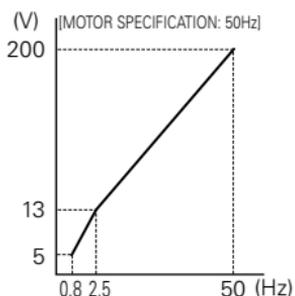
When operating with frequency larger than 60Hz/50Hz, change only max. output frequency (n011).
