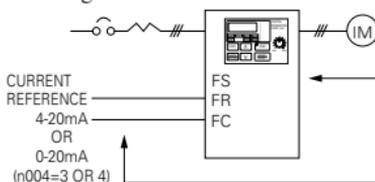
Press the digital operator keys to run or stop the inverter. Switch run and stop direction by setting F/R LED.
