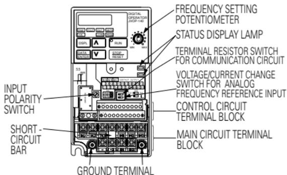
Example of 3-phase (200V class, 0.1kW) inverter
