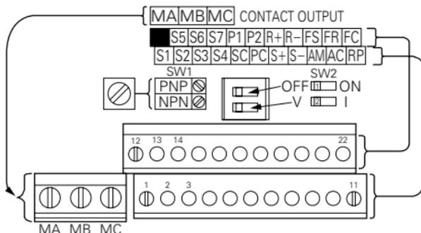
\* SW1 can be changed according to sequence input signal (S1 to S7) polarity.
