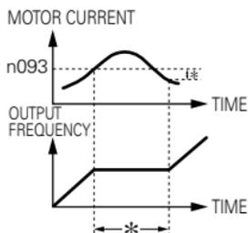
\*Stops the acceleration to prevent the motor from stalling.
