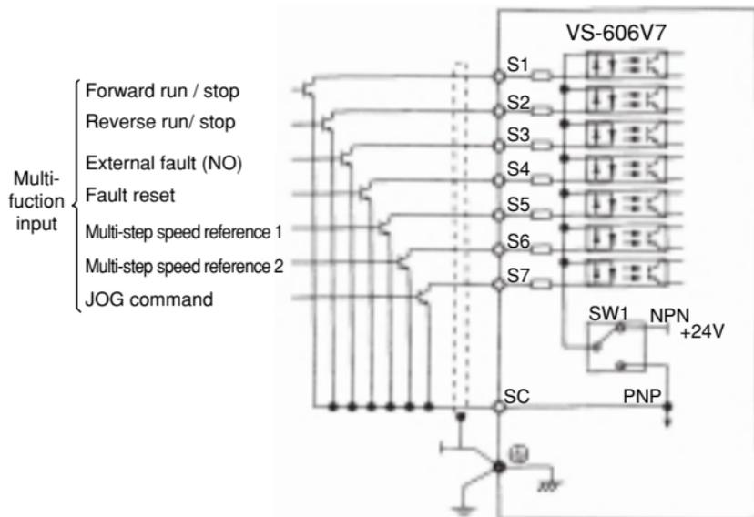
Sequence connection with PNP transistor (+24V common)
