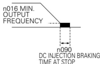
When coasting to a stop is specified in stopping method selection (n005), DC injection braking at stop does not operate.
