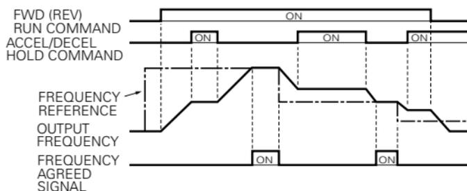
Note : When the FWD (REV) run command is input along with the accel/decel hold command, the motor does not operate. However, when frequency reference lower limit (n034) is set greater than or equal to min. output frequency (n016), the motor operates at frequency reference lower limit (n034).
