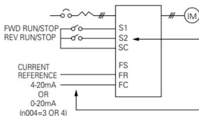
Switch run/stop and FWD/REV run with switching device connected to the control circuit terminal.
