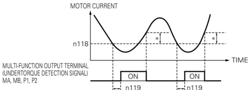
\* Undertorque detection release width (hysteresis) is set at approx. 5% of the inverter's rated current.
