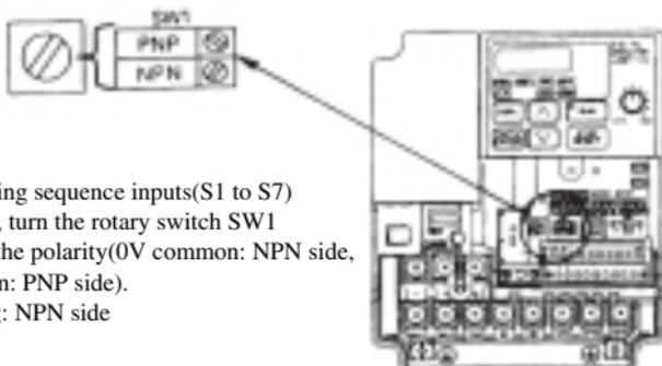
When connecting sequence inputs(S1 to S7) with transistor, turn the rotary switch SW1 depending on the polarity(0V common: NPN side, +24V common: PNP side).
