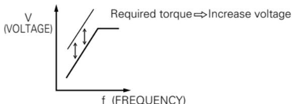
Normally, no adjustment is necessary for torque compensation gain (n103 factory setting : 1.0). When the wiring distance between the inverter and the motor is long, or when the motor generates vibration, change the automatic torque boost gain. In these cases, set the V/f pattern (n011 to n017).
