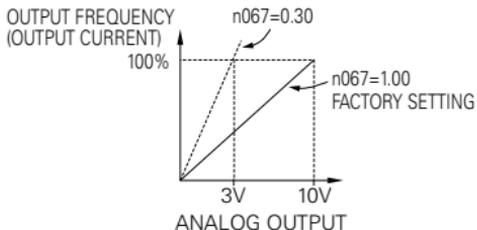
Set the analog output voltage at 100% of output frequency (output current). Frequency meter displays 0 to 60Hz at 0 to 3V.
