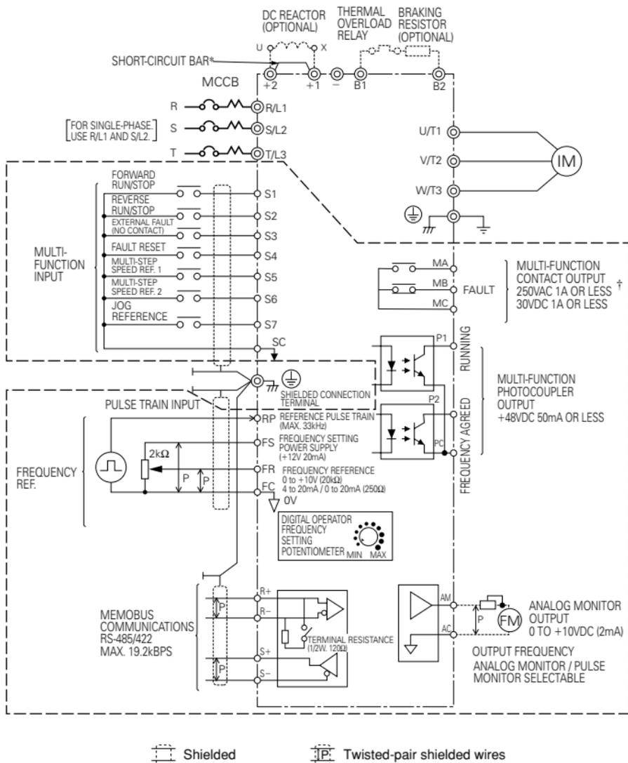
[---]: Only basic insulation (Protective class 1, overvoltage category II) is provided for the control circuit terminals. Additional insulation may be necessary in the end product to conform to CE requirements
