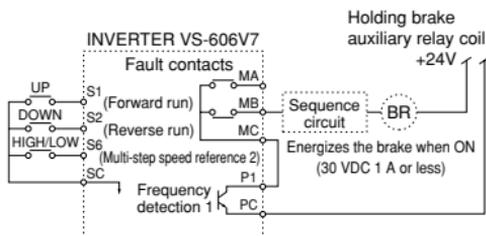
For the AC sequence circuit, connect the signal between P1 and PC to the sequence circuit with a relay.
