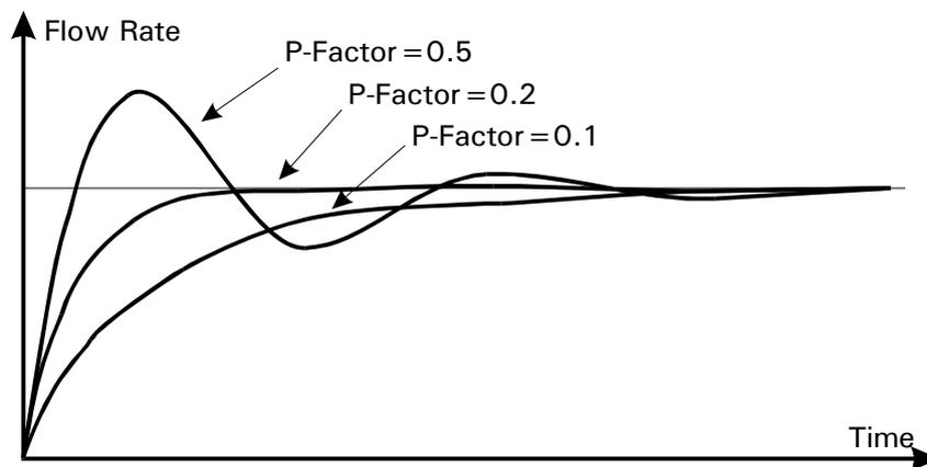
Damping of P-controller by adding a D-component:
