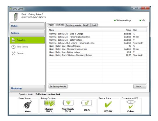
For each of the following conditions, both a warning and an alarm threshold value can be defined:
