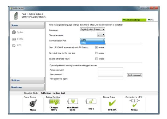
If you click the combo box near the text "Communication port" the correct port is shown and you can select it.
