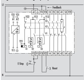
The single channel fulfills the requirements of EN 60204-1. However the circuit of the E-Stop is not redundant. Ground faults in the circuit for the E-Stop contact are detected.
