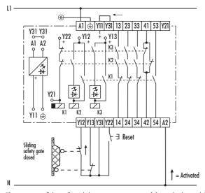
The position of the safety sliding gate is monitored through channel 1 (Y12) and channel 2 (Y13). The SNO 1002 is activated through the RESET switch. If the sliding safety gate opens, the E-Stop Safety Relay returns to its off-position and the enabling current paths 13/14, 23/24, 33/34 open. If the safety gate is closed again the E-Stop Safety Relay can be activated again through the RESET switch.
