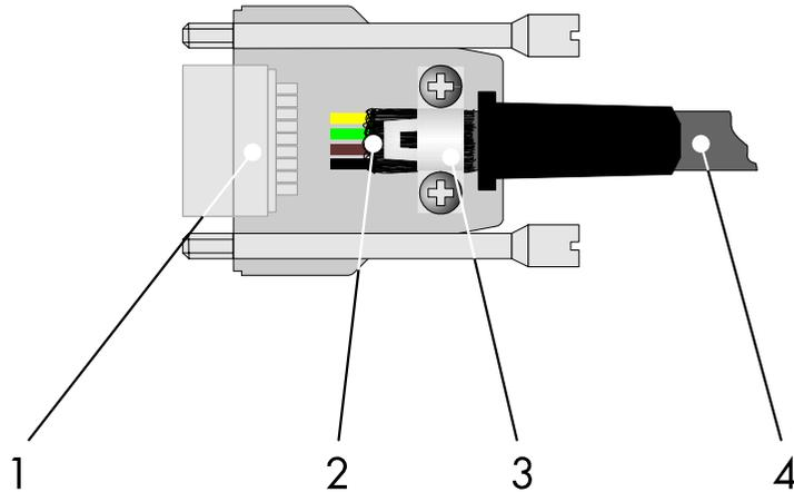
Figure A-1 Shielding D-SUB connectors
