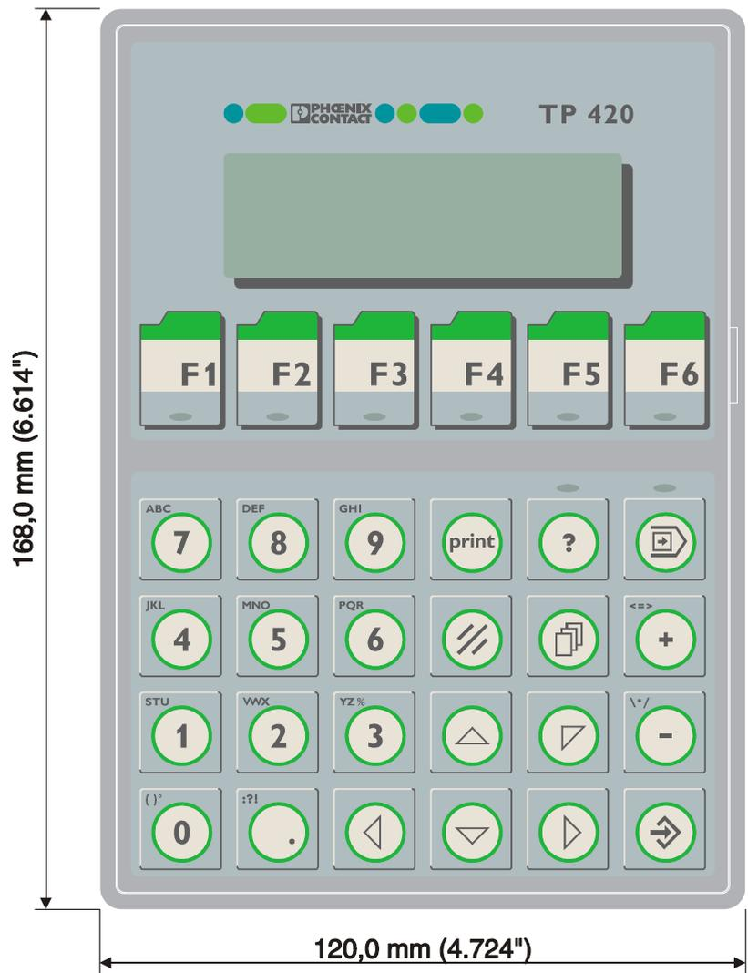
Figure 1-7 Dimensions of the front plate
