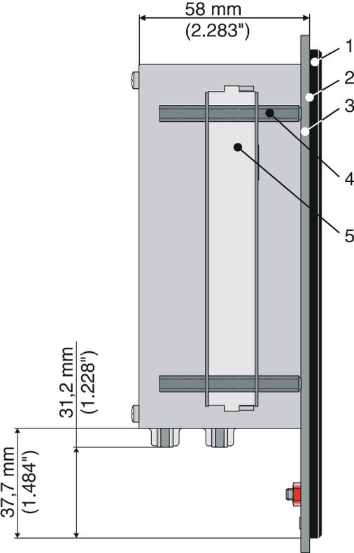
Figure 1-8 Side view, installation depth
