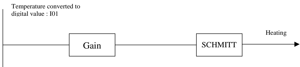
Fig. 1.55 Logic diagram for temperature control.
