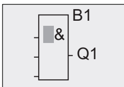
The AND is the first block of the basic functions list. The solid square cursor prompts you to select a block.
