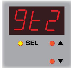
**gt2** is displayed. Press the **SEL** button and use the ▲ and ▼ buttons to select the second three digits of the gateway address. Press the **SEL** button again.
