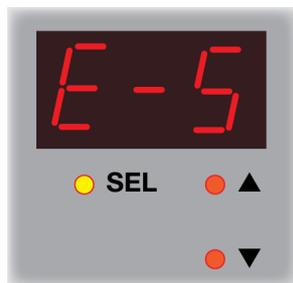
Use the ▲ and ▼ buttons to select **E-5** to enter values from 0.02ms to 9.98ms in steps of 0.02ms using a PP520 or 0.01ms to 9.99ms in steps of 0.01ms using a PP520F.
