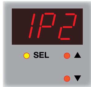
**IP2** is displayed. Press the **SEL** button to read the second three digits of the IP address.
