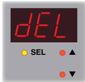
**deL** is displayed. Press the **SEL** button to set up the delay time as described in [Section 9.6, Setting pulse delay and width times](#).
