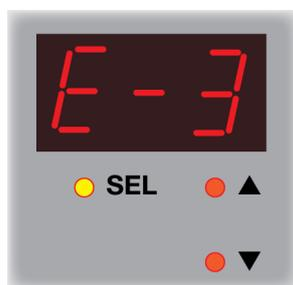
Use the ▲ and ▼ buttons to select **E-3** to enter values from 1ms to 999ms in steps of 1ms. Press the **SEL** button.
