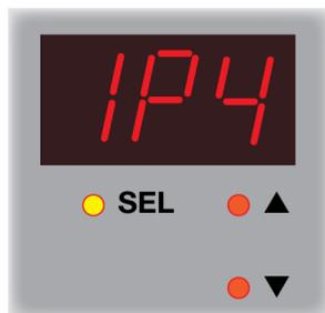
**IP4** is displayed. Press the **SEL** button and use the ▲ and ▼ buttons to select the fourth three digits of the IP address. Press the **SEL** button again.
