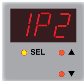
**IP2** is displayed. Press the **SEL** button and use the ▲ and ▼ buttons to select the second three digits of the IP address. Press the **SEL** button again.
