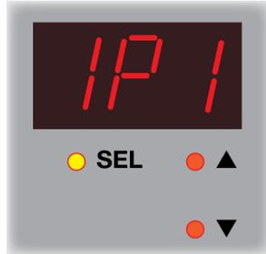
**IP1** is displayed. Press the **SEL** button and use the ▲ and ▼ buttons to select the first three digits of the IP address. Press the **SEL** button again.
