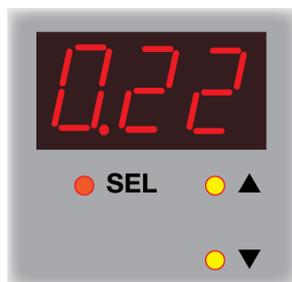
Use the ▲ and ▼ buttons to select the rating of the light in Amps. The current is adjustable in steps of 10mA. Press the **SEL** button when you have set the current.
