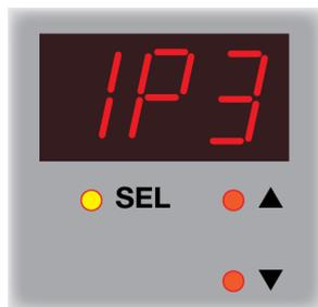
**IP3** is displayed. Press the **SEL** button and use the ▲ and ▼ buttons to select the third three digits of the IP address. Press the **SEL** button again.
