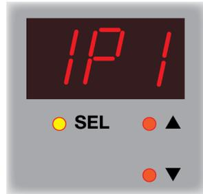
**IP1** is displayed. Press the **SEL** button to read the first three digits of the IP address.
