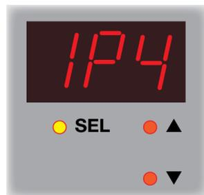
**IP4** is displayed. Press the **SEL** button to read the remaining digits of the IP address.
