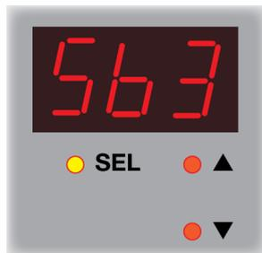
**Sb3** is displayed. Press the **SEL** button and use the **▲** and **▼** buttons to select the third three digits of the subnet mask. Press the **SEL** button again.
