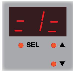
The PP520 displays a pattern of alternating horizontal bars when the light is operating normally. If you power cycle the controller, it will resume with the same settings.
