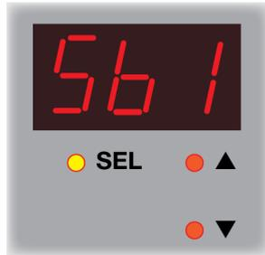
**Sb1** is displayed. Press the **SEL** button and use the **▲** and **▼** buttons to select the first three digits of the subnet mask. Press the **SEL** button again.
