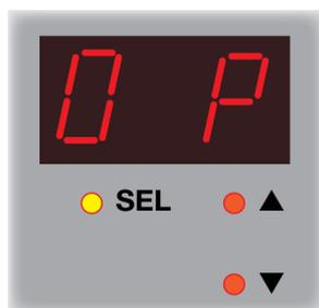
If an error occurs (if the light is disconnected for example), the PP520 displays **OP**. Press the **SEL** button to cancel this.
