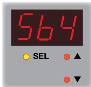
**Sb4** is displayed. Press the **SEL** button and use the **▲** and **▼** buttons to select the fourth three digits of the subnet mask. Press the **SEL** button again.
