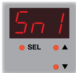
When the PP520 detects a light connected to channel 1 for the first time, **Sn1** is displayed. (A light connected to channel 2 will display **Sn2**).
