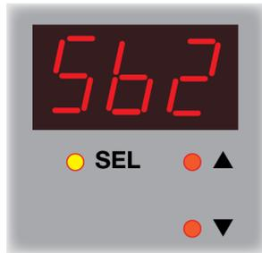
**Sb2** is displayed. Press the **SEL** button and use the **▲** and **▼** buttons to select the second three digits of the subnet mask. Press the **SEL** button again.
