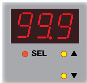
Use the ▲ and ▼ buttons to set the intensity from 1% to 99.9%, and press the **SEL** button.
