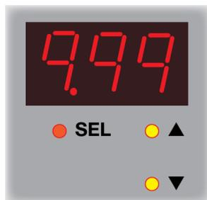
Use the ▲ and ▼ buttons to select the desired value. Press the **SEL** button.
