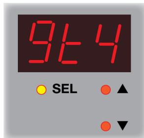
**gt4** is displayed. Press the **SEL** button and use the ▲ and ▼ buttons to select the fourth three digits of the gateway address. Press the **SEL** button again.
