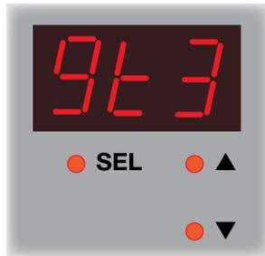
**gt3** is displayed. Press the **SEL** button and use the ▲ and ▼ buttons to select the third three digits of the gateway address. Press the **SEL** button again.
