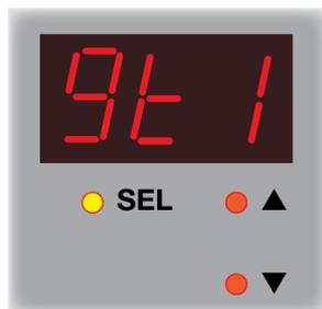
**gt1** is displayed. Press the **SEL** button and use the **▲** and **▼** buttons to select the first three digits of the gateway address. Press the **SEL** button again.
