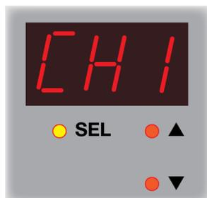
**CH1** is displayed. Use the ▲ and ▼ buttons to select **CH2** if you wish to set up channel 2. Press the **SEL** button.
