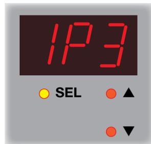
**IP3** is displayed. Press the **SEL** button to read the third three digits of the IP address.
