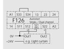
Activation as well as supply via 24Vpc semiconductoroutputs (without activation of the "Power LED"); Automatic reset
