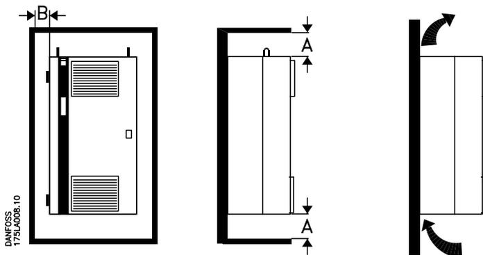
Please note that the frequency converter can be installed without any free space to the sides; however, the hinges must be able to move freely; (Distance B).
