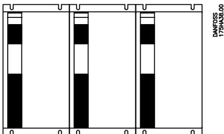
VLT 3500 HVAC can be installed with the flanges side by side.
