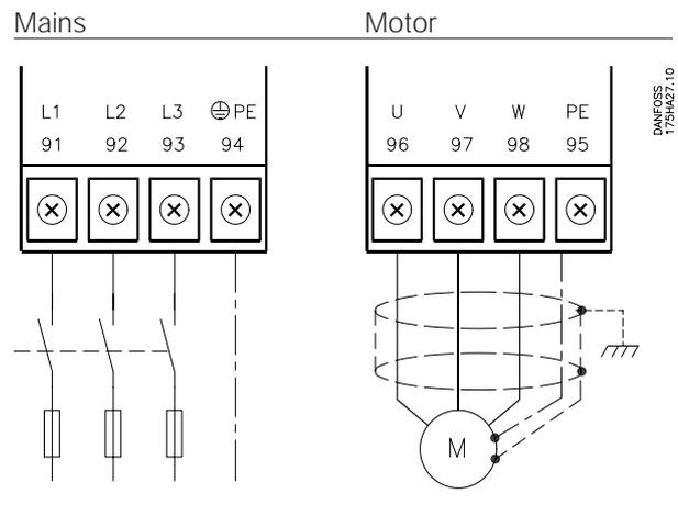
■ Mains and motor connection of VLT 3575-3600 HVAC and VLT 3542-3562 (230 V) HVAC
