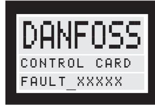
The reason for this fault message is a fault on the control card or an option card, if used. Contact DANFOSS.
