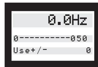
**Stop Reset** This key is used to stop the connected motor. If stop is activated, the top line in the display will start to flash. The key on the operating panel of the frequency converter does not turn off the mains supply and is thus not to be used as a safety switch.
