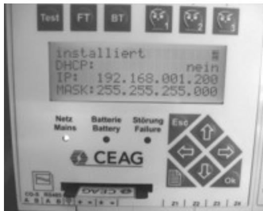
The webmodule gets automatically activated to the control unit, which is displayed by the red LED (some seconds) of the control unit and the webmodule. After 1-2 minutes the procedure is finished and the webmodule is ready to operate.
