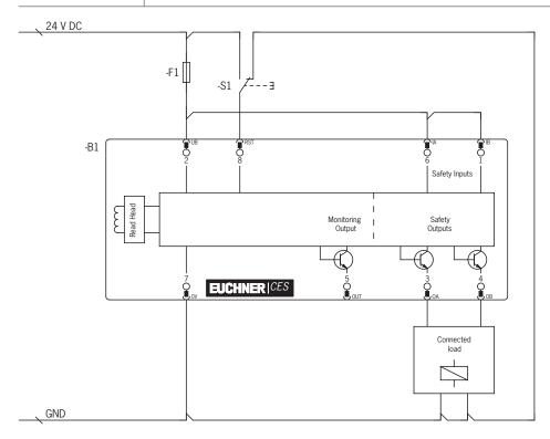
Figure 3: Connection example for separate operation of a CES-AR-...
