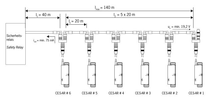
Figure 1: Circuit example with six CES-AR
