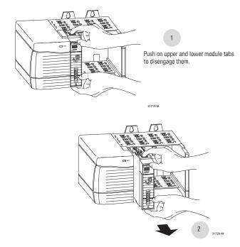
Slide module out of chassis.
