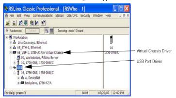
Your module appears under two different drivers, a virtual chassis and the USB port. You can use either driver to browse through your 1756-DNB scanner module.
