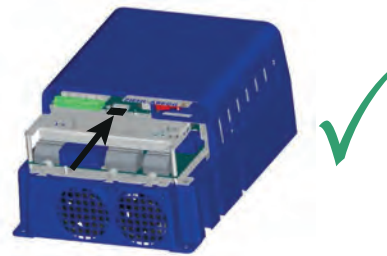
Memory card in the X-MMC card slot of ZAdyn4C 011-032
