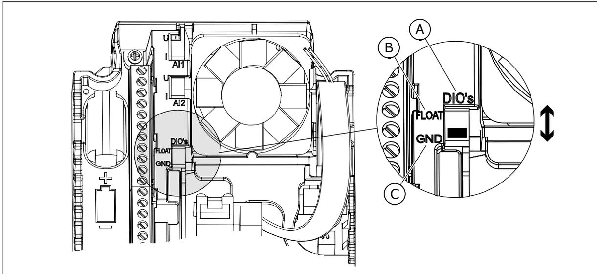
Fig. 30: Change the position of this switch to isolate the digital inputs from ground
