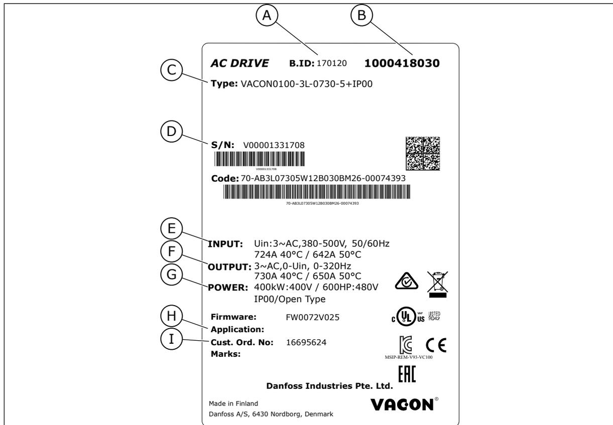
Fig. 2: The package label of VACON® AC drives
