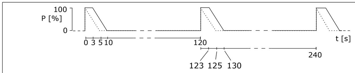
Fig. 36: The duty cycles of the LD and HD pulses
