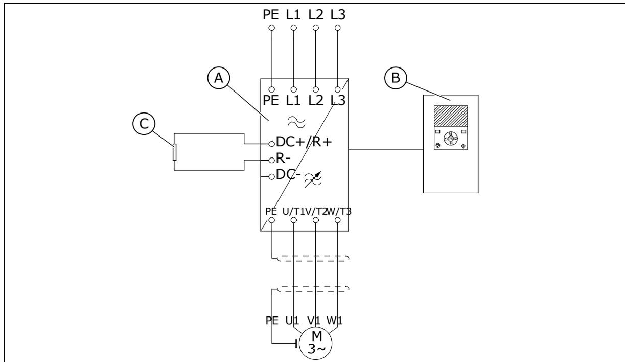
Fig. 12: The main circuit diagram, MR8 and MR9
