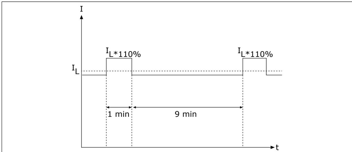
Fig. 37: Low overload in VACON® 100 FLOW
