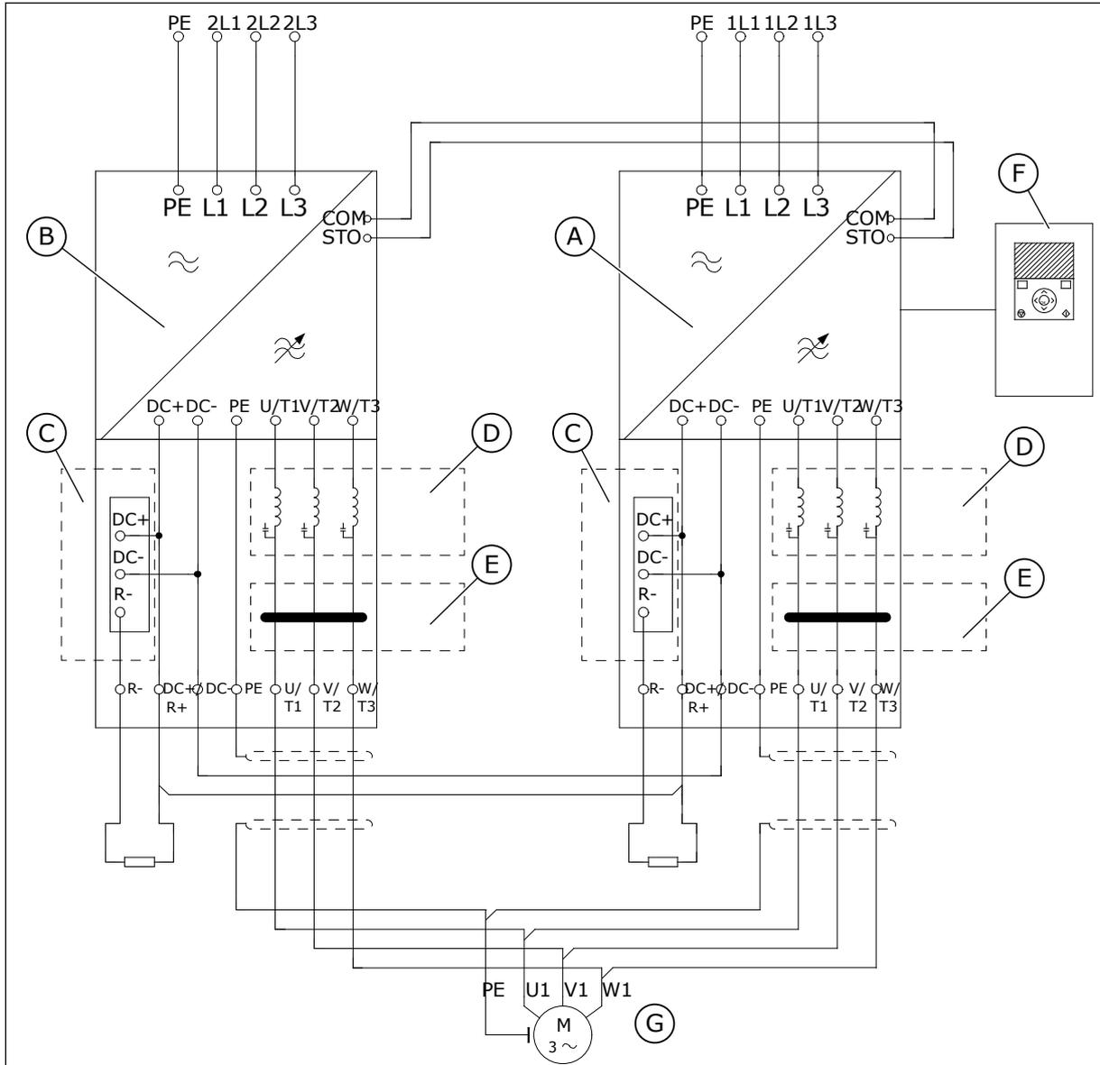
Fig. 16: The main circuit diagram, MR12 with the options module and options
