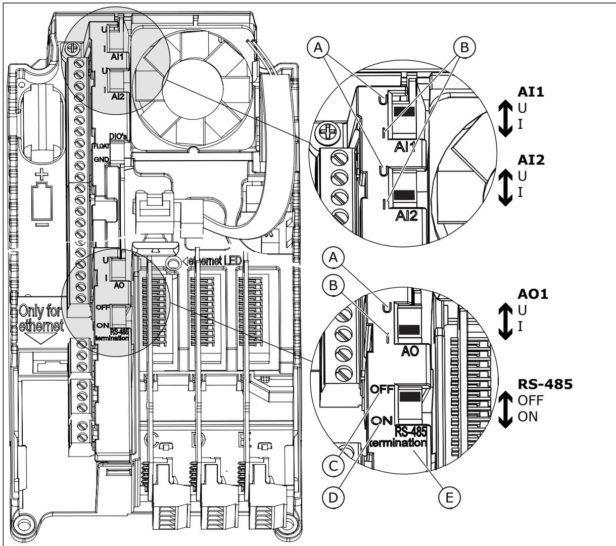
Fig. 29: The selections of the DIP switches
