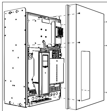
2 MR9 only: Loosen the screws and remove the sealing plate.
