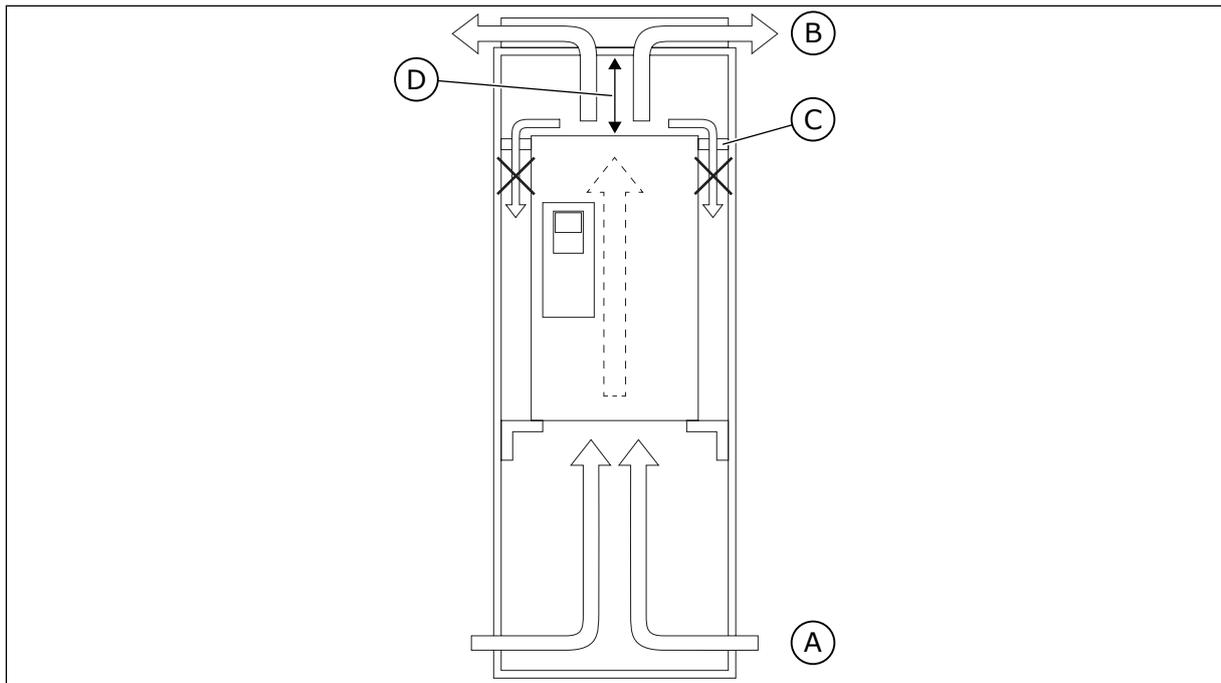
Fig. 21: The correct circulation of cooling air inside the cabinet
