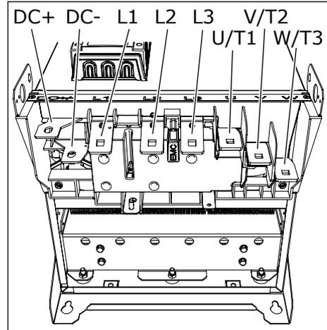
2 In MR12, connect the DC terminals of the 2 power units with the DC link cable. Connect the DC+ terminals together, and the DC- terminals together. The DC link cable is included in the delivery.
