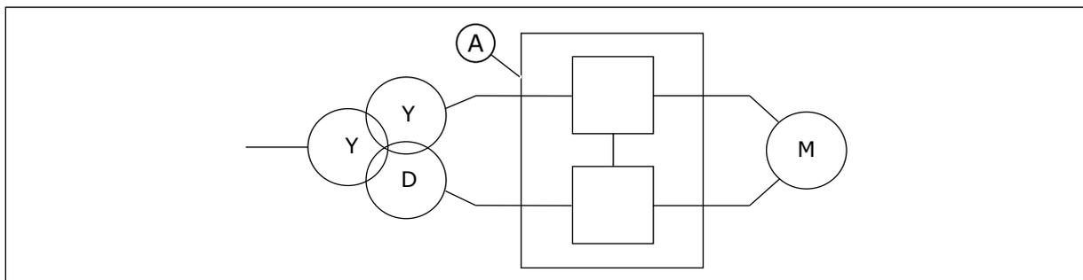
*Fig. 17: The 12-pulse operation of MR12*
