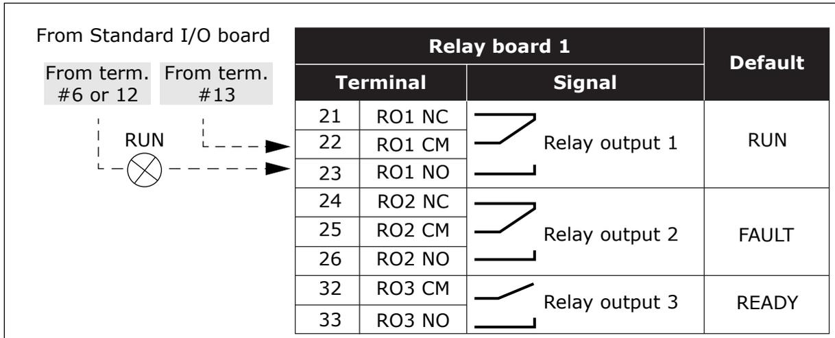
Fig. 27: The standard relay board (+SBF3)
