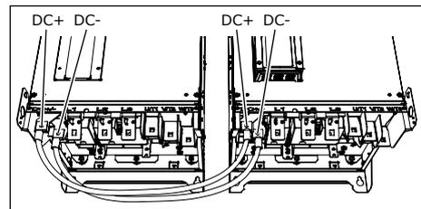
3 Use the external power connection block (+PCTB) if you have it. For MR12 there are 2 external power connection blocks.
