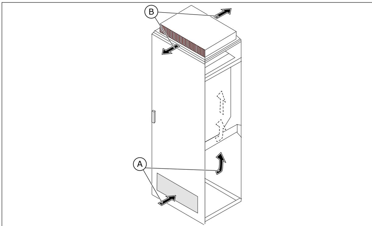
Fig. 22: The cooling air must move freely inside the cabinet
