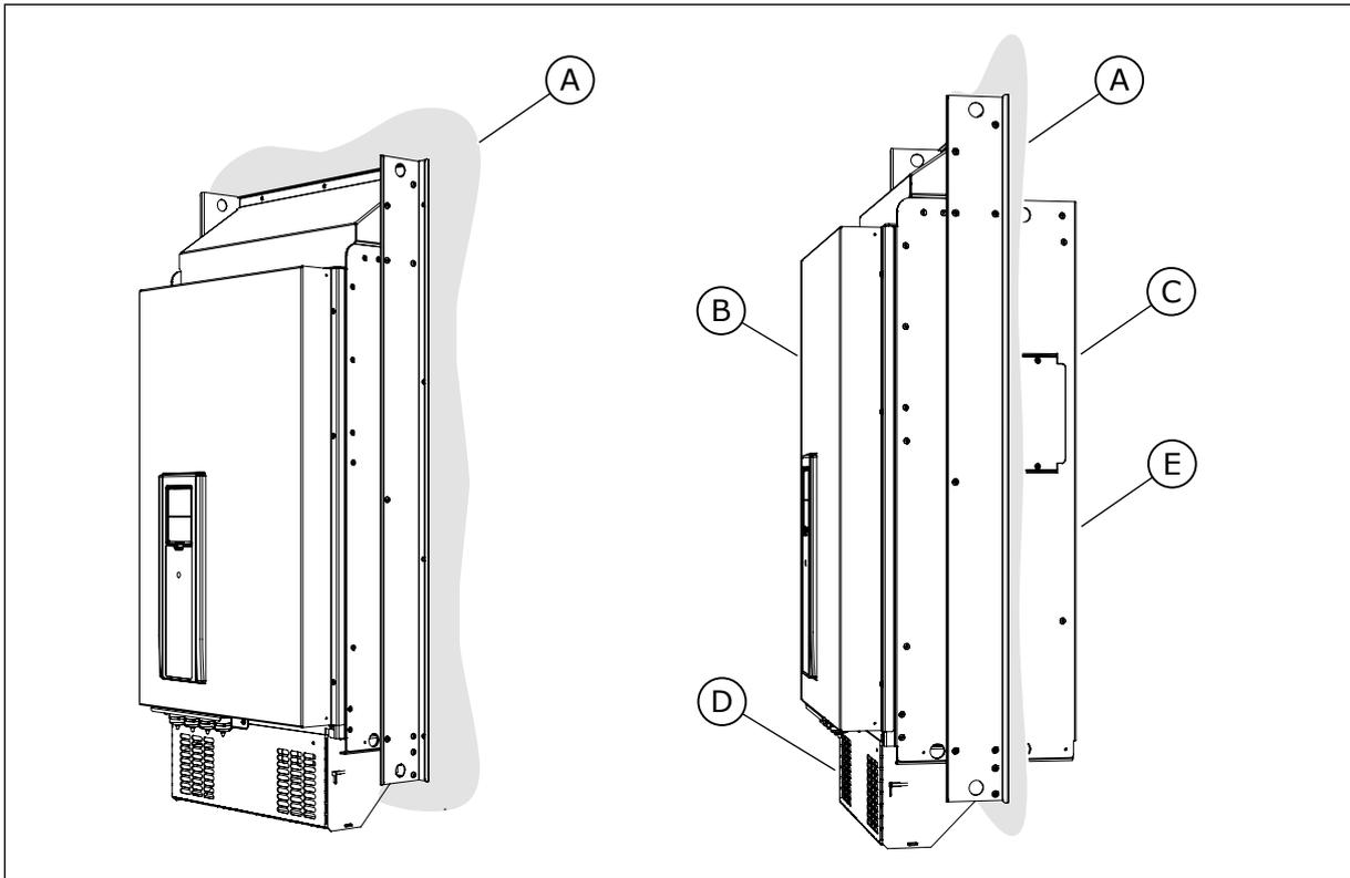
Fig. 18: Example of flange mounting (enclosure size MR9)
