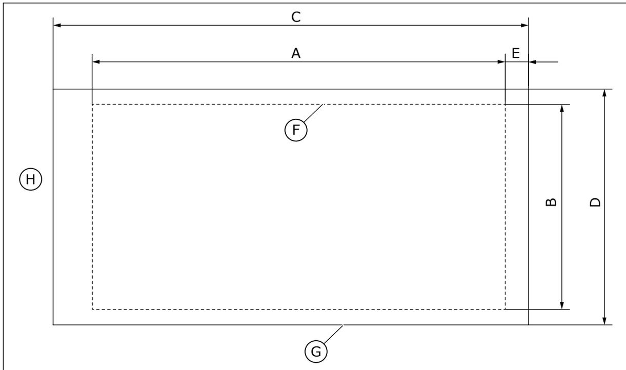
Fig. 19: The dimensions of the opening and drive module outline with flange
