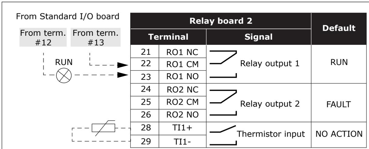
Fig. 28: The optional relay board (+SBF4)
