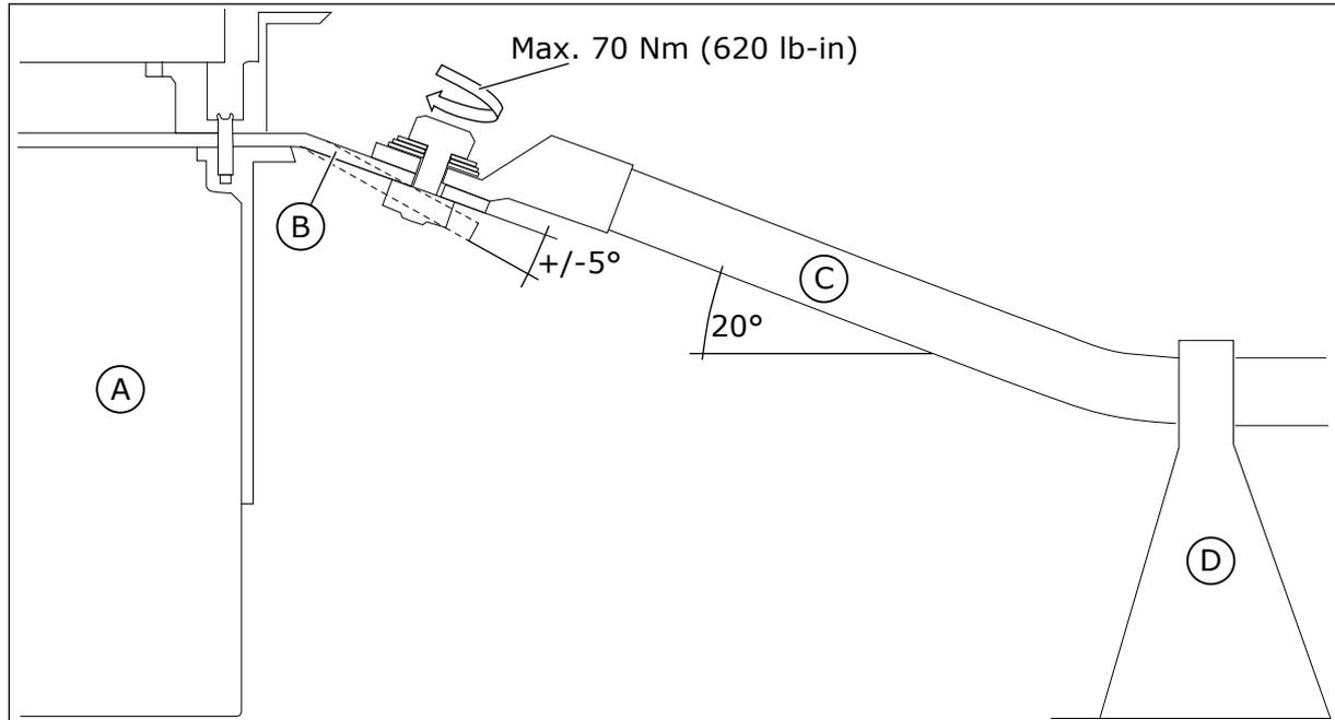
Fig. 24: Mechanical support for cables when the drive does not have the options module
