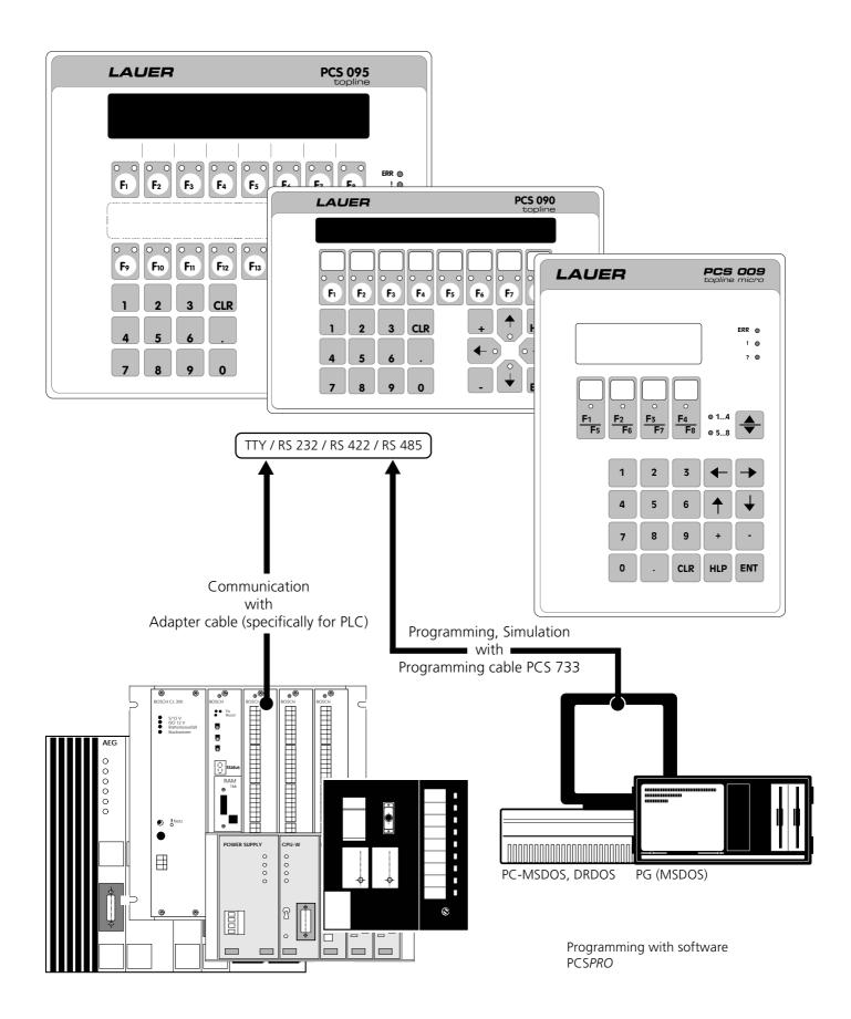
PCS is a universal operating concept for many PLC systems. The operating panels PCS 009, PCS 090, PCS 095, PCS 095.1 have a large selection of ready-made functions and tools to operate and monitor with:
