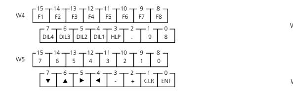
These key bits are log 1, so long as the respective key is pressed and the communication runs without fault. The control keys in the LOW byte of W5 should only be used with care, as they are also required for the editing of nominal values in several priorities, especially in the menu priority for editing.
