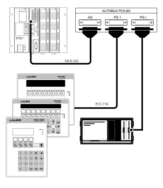
The Automux PCS 809 removes this problem. The PCS 809 broadens the PLC-PG-interface so that the PG and the PCS can serve the PLC together. The switch over to MUX follows automatically.
