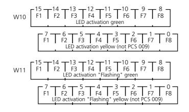
A green and a yellow LED (not for PCS 009)per function key F1...F8 is available. Every LED can take on 4 conditions, as each LED has 2 bits at its disposal:
