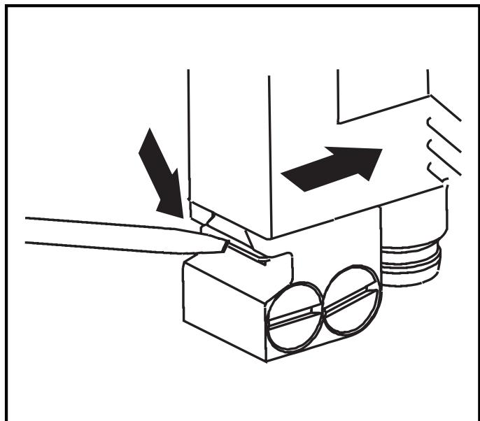
To remove the unit press the spring down with a screwdriver and slide the unit out.
