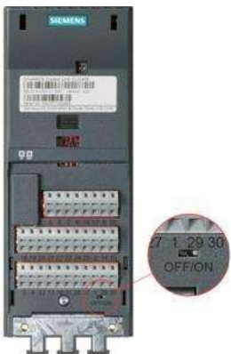
Fig. 4 – DIP switch for bus termination on CU240E
