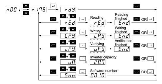
**Note** The following display is an example of the capacity displayed. The values in parentheses indicate the capacities for European motors.
