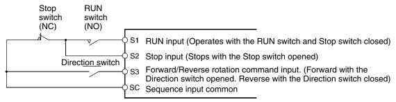
Note Set parameter 052 to forward/reverse rotation command 0 for 3-wire sequence input.
