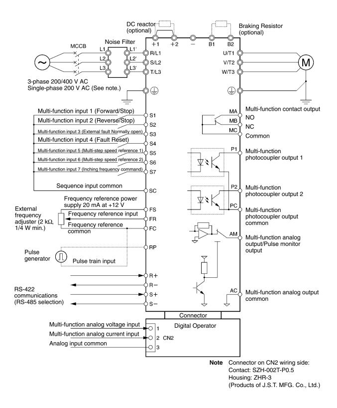
**Note** Connect single-phase 200 V AC to terminals R/L1 and S/L2 of the 3G3MV-AB.
