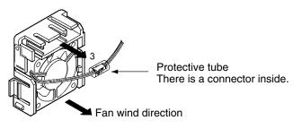
3. Slide the protective tube and remove the internal connector.
