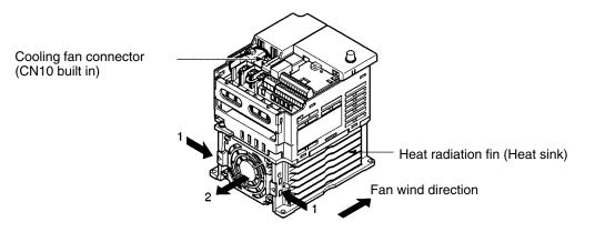
2. Press the left and right sides of the fan cover located on the lower part of the radiation fin in the arrow 1 directions. Then lift the bottom of the Fan in the arrow 2 direction to remove the fan as shown in the following illustration.
