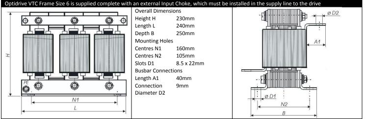
Note: The choke is always supplied with the drive, and MUST be used.
