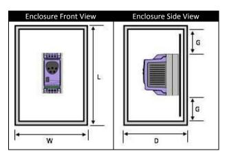
The enclosure design and layout should ensure that the adequate ventilation paths and clearances are left to allow air to circulate through the drive heatsink. Invertek Drives recommend the following minimum sizes for drives mounted in non-ventilated metallic enclosures:-
