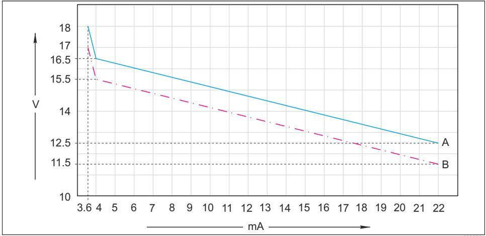
Fig. 11: Minimum supply voltage at the transmitter depending on the output current
