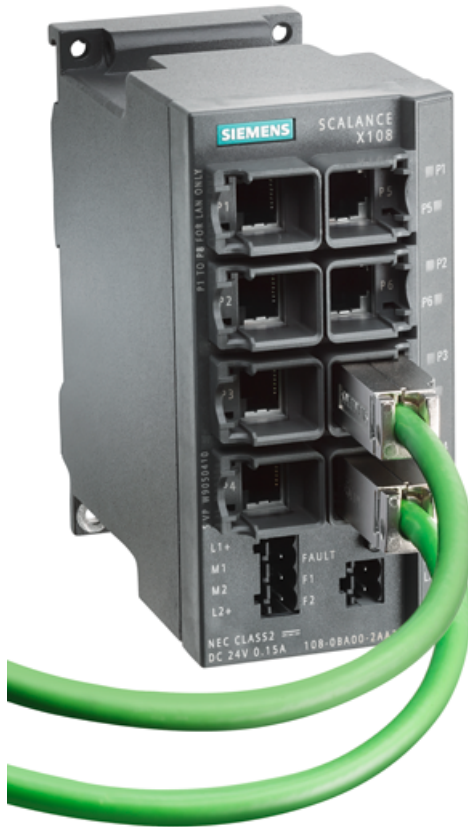
Figure 6-2 Plugging in the IE FC RJ45 Plug 180
