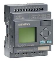
\*\*\* Spare part \*\*\* LOGO! 12/24RC, logic module, displ. PS/I/O: 12/24 V DC/relay, 8 DI (4 AI)/4 DO, memory 200 blocks, modular expandable
